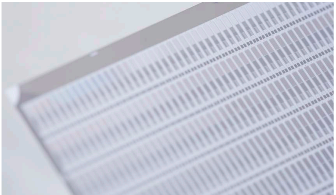
Sensor substrate after passing through clean room processes.
