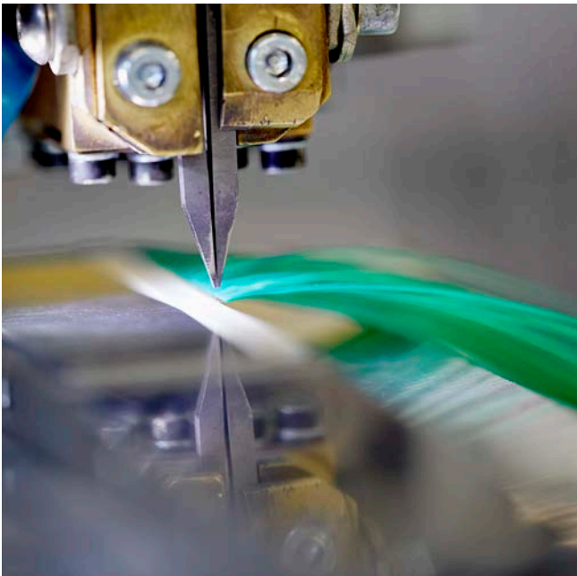
Welding of wires to the sensor
